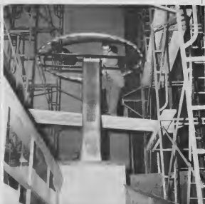
RECENTLY installed in the General Assembly Building of the United Nations in New York is this Foucault Pendulum. As the ball (visible behind left side of dial ring) swings back and forth, the dial rotates on its axis.
